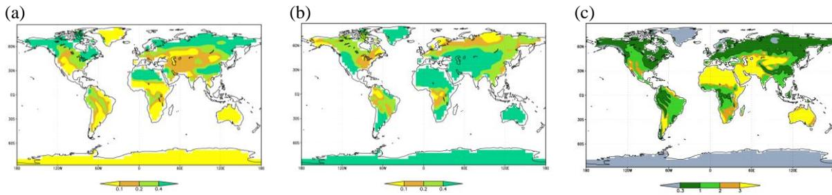
Figure 2. Simulated long term mean rainfall-runoff chain (Global Climate Model ECHAM5 20C): Geographical distributions of (a) excess water  $W$  (runoff-rainfall ratio), (b) excess energy  $U$ , and (c) dryness ratio  $D$ .
