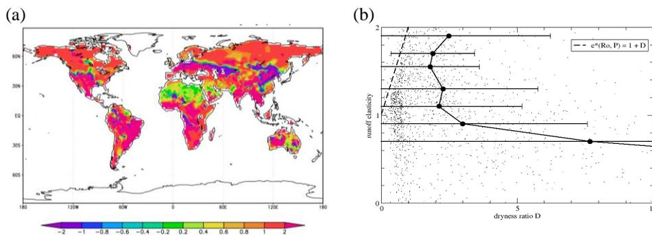
Figure 5. Rainfall induced runoff elasticity  $\varepsilon(Ro, P)$  simulated by ECHAM5 20C: (a) Geographical and (b) dryness  $D$  dependent distributions (scatter plot); runoff elasticity  $\varepsilon^*$  based on Schreiber's formula (dashed).
