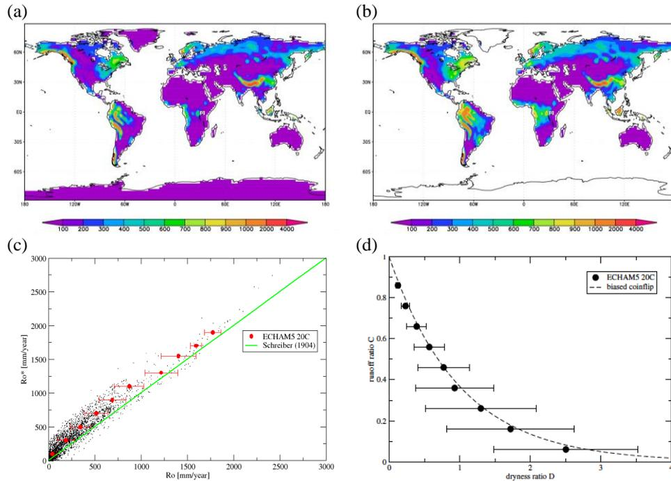
Figure 4. Validation of the rainfall–runoff chain: The geographical distributions of mean streamflow (a)  $Ro$  simulated (ECHAM5 20C), and (b)  $Ro^*$  derived by Schreiber's formula using simulated dryness  $D$  and rainfall  $P$ , are (c) compared in a ( $Ro$ ,  $Ro^*$ )-scatter plot. (d) GCM-simulated dryness  $D$  and excess rainfall  $W$  sampled in  $W$ -bins (means, standard deviations as dots, horizontal lines) align Schreiber's formula (dashed).
