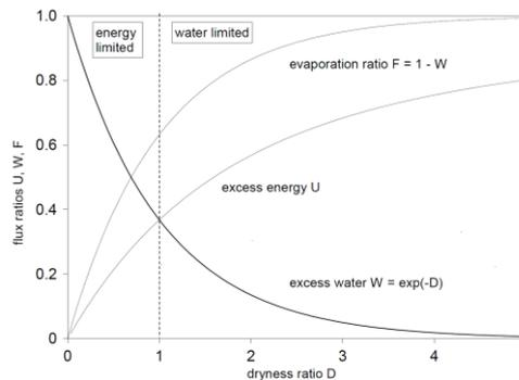
Figure 1. Idealized long term mean rainfall-runoff diagram (Schreiber 1904): Functional relation of excess water  $W$  (runoff-rainfall ratio) and excess energy  $U$  depending on dryness ratio  $D$ ; evaporation ratio  $F$  is also included.
