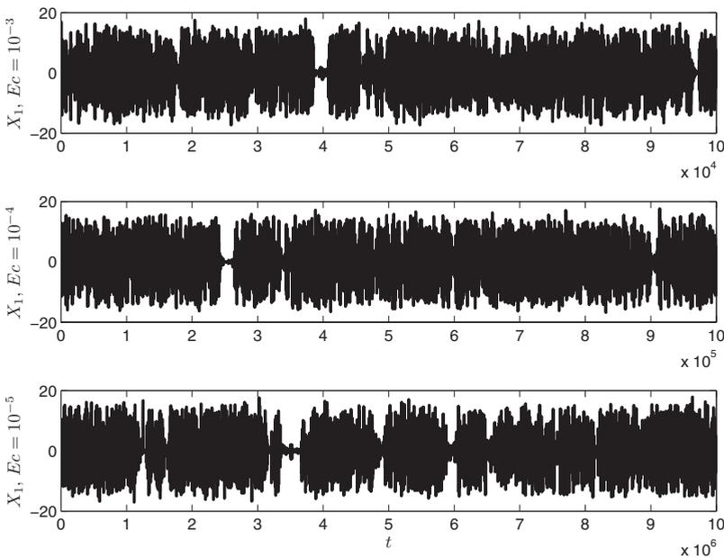
FIG. 3. Impact of the viscous-thermal feedback on the time scales of the system. From top to bottom: typical evolution of the variable  $X_1$  for different values of the Eckert number ( $Ec=10^{-3}$ ,  $Ec=10^{-4}$ , and  $Ec=10^{-5}$ , respectively). Note that the time scale is magnified by a factor of 1, 10, and 100 from top to bottom. Details in the text.
