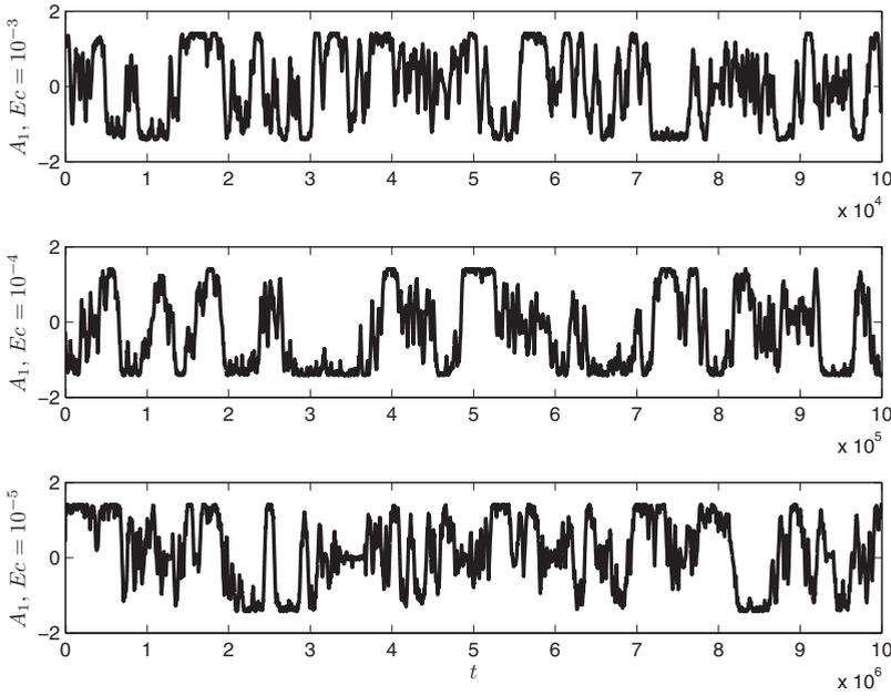
FIG. 2. Impact of the viscous-thermal feedback on the time scales of the system. From top to bottom: typical evolution of the variable  $A_1$  for different values of the Eckert number ( $Ec=10^{-3}$ ,  $Ec=10^{-4}$ , and  $Ec=10^{-5}$ , respectively). Note that the time scale is magnified by a factor of 1, 10, and 100 from top to bottom. Details in the text.
